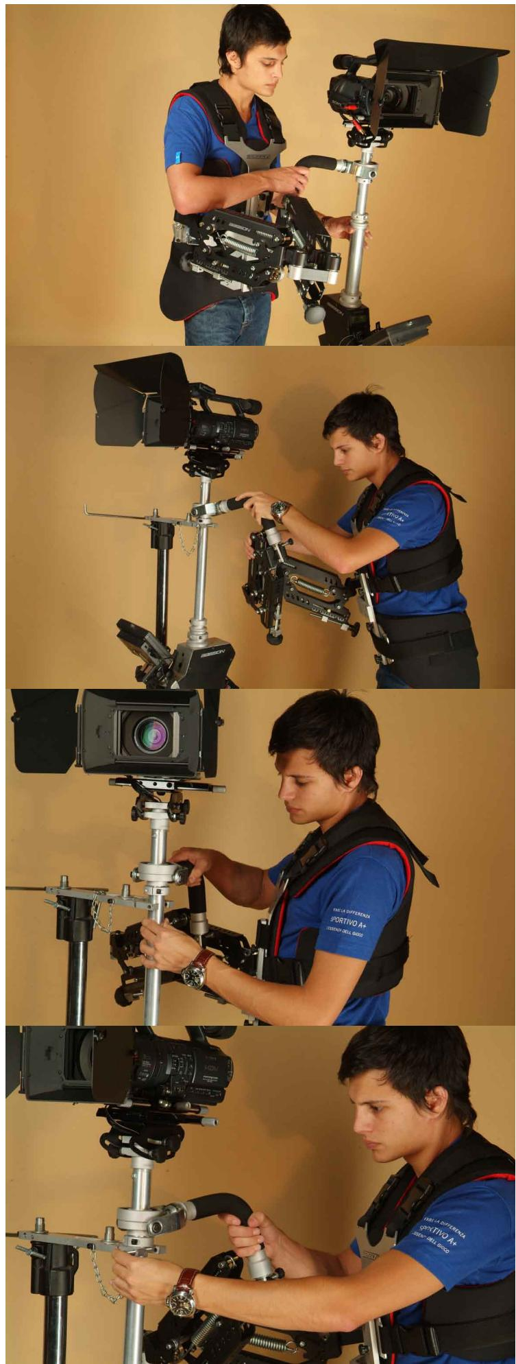
**The arm tension is adjusted for the heaviest camcorder it can hold so it does not bottom out when you put the camcorder and sled on the arm for the first time. Now adjust the arm for the weight of your camcorder:**
